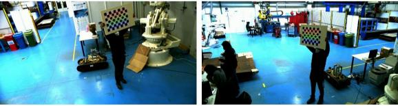
Figure 2. Example of images captured for stereo calibration.
