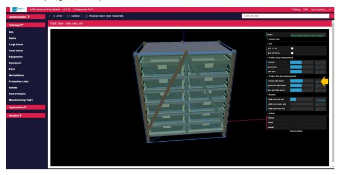
5.3. Once the CAD model is aligned with the Bounding Volume, press Update button to save the configuration. A message is presented "The configuration is up to date" confirming the action.
