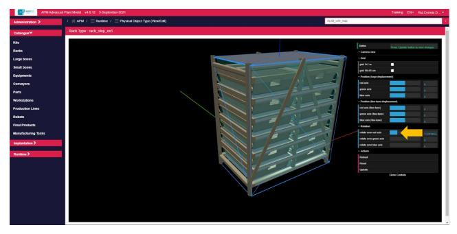
5.2. Adjust CAD model **location** using the **Position sliders**. Each slider performs a translation over a specific axis (red, green, or blue).
