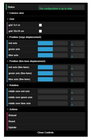
5.1. Adjust CAD model **orientation** using the **Rotation sliders**. Each slider performs the rotation over a specific axis (red, green, or blue).
