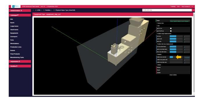
5.2. Adjust CAD model **location** using the **Position sliders**. Each slider performs a translation over a specific axis (red, green, or blue).
