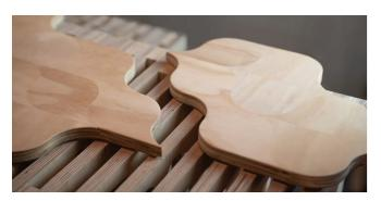
An open-source Grasshopper tool that parametrically creates shapes out of the leftover sheet material from CNC frasing. It demonstrated a 70% + reduction of material waste & CO2 emissions compared to standard CNC nesting solutions, 20% less sheets needed for equal output and created an open workflow allowing collaborating with external designers. Hence, contributing to creativity and sustainability.
