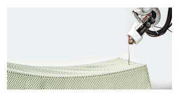
An algorithm allowing the creation of large-scale 3D printed objects mimicking crochet or willow weaving. It reduces printing time by 50% due to open woven structures, opens up a new area of 3D printing possibilities using less material than solid structures and makes it possible to use 3rd life (or 3x recycled) waste. Hence, contributing to efficiency and sustainability for the company and region.
