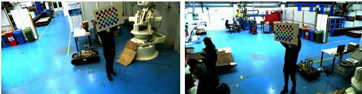
*Figure 2. Example of images captured for stereo calibration.*
