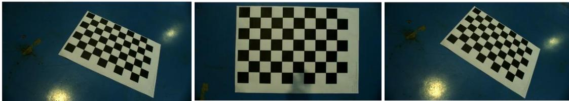
*Figure 1. Example of images captured for individual calibration.*
