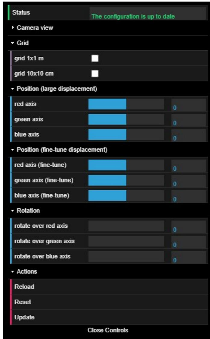
5.1. Adjust CAD model **orientation** using the **Rotation sliders**. Each slider performs the rotation over a specific axis (red, green, or blue).
