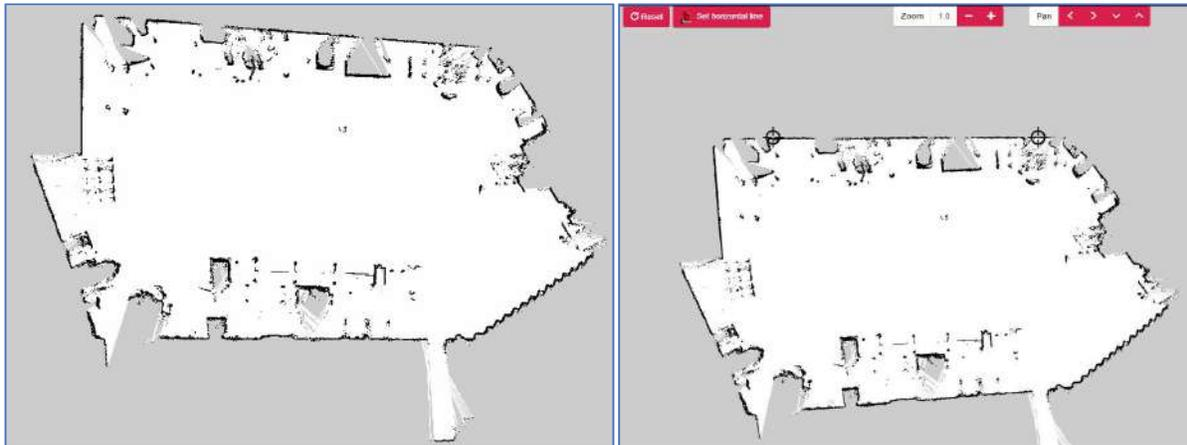
Figure 23 – Implantation: Map non-horizontally aligned (on the left) and horizontally aligned (on the right)
